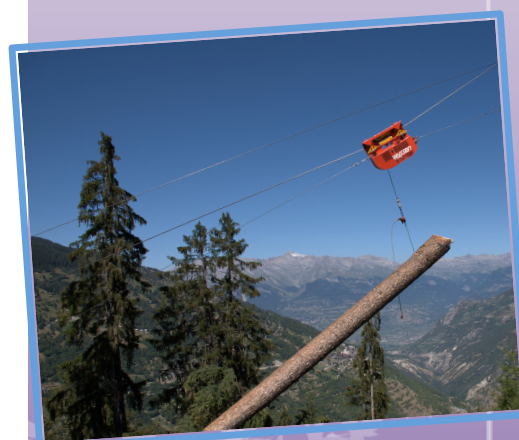
"Carriage" used to lift and move trees
